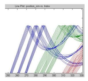
You now have some idea how damping has affected the test results. You have a cluster of blue, green, and red indicating that damping is the same value in each cluster, which you can confirm by using the test selection tool to choose lines and by viewing the value for the Damping test vector in the **Current Iteration** pane.
