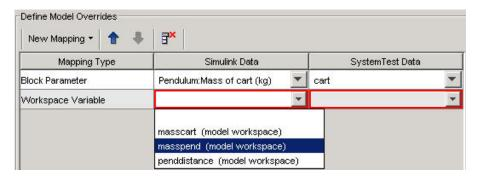
**3** Specify which SystemTest test vector or test variable you want to map to the Simulink workspace variable. Click the **SystemTest Data** field of this row to see all available test vectors and test variables. For this example, select **pend**.
