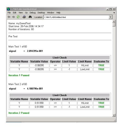
The Main Test section of the test execution log shows each iteration. You see the value of the test vector signal and determine the values the Limit Check element used in evaluating whether the test passed. For the first several iterations, the value of Y did not exceed either the high or low limits so the iterations passed. You can also see this in the scalar plot drawn while the test ran. For other iterations that failed, you can scroll through the test execution log to find the values of Y.
