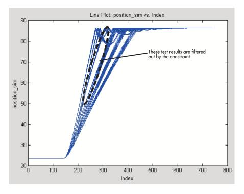
If you change the value of the constraint to 1 using the slider, you will show only those test results that passed the Limit Check element in your test.
