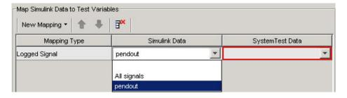
3 Specify the SystemTest test variable to which you want to map the output. Click the SystemTest Data field and select a test variable. For the Inverted Pendulum example, select st\_loggedsignal.
