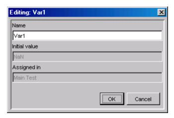
**8** Enter a name for the test variable, such as DUTresponse, then click  $\mathbf{OK}$  to create the test variable.
