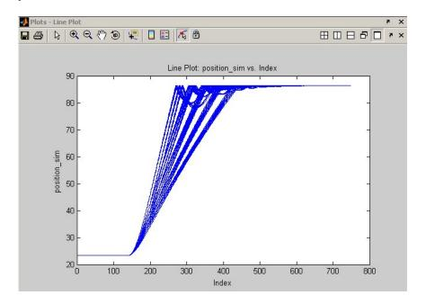
Each line in the plot represents a test iteration. If it appears that there are not as many lines as you had test iterations, it is possible that two or more iterations generated similar enough results that they overlap.
