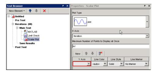
With each Main Test iteration of the test, the Scalar Plot element updates a figure window with data you selected.
