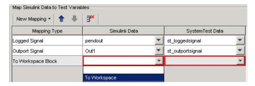
**3** Specify the SystemTest test variable to which you want to map the To Workspace block. Click the **SystemTest Data** field and select a test variable from the list. For this example, select **New Test Variable** to create a test variable.
