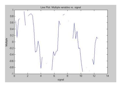
You can just as easily show only the iterations of your test that failed by reconfiguring the constraints you created to filter out data that is < -1 or > 1. Alternatively, you can create a new constraint that uses a MATLAB expression. For example:
