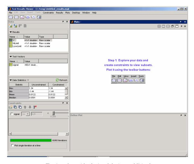
The viewer has a rich selection of plotting capabilities that you can use to visualize your test results. Plotting capabilities include line, scatter, time series, surf, waterfall, and image plots. Using the signal example, you can reproduce the line plot that your scalar plot element generated during the test.
