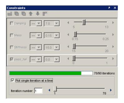
The **Constraints** pane changes to show a slider and the currently displayed test iteration.
