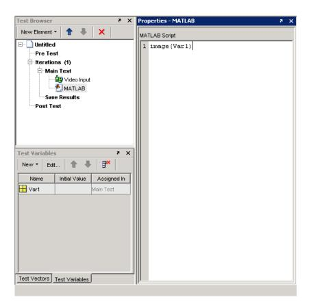
This completes this example test illustrating how to incorporate image data into SystemTest. In a real testing application, you can define test vectors that determine the number of iterations of your test that SystemTest performs. You can also compare test variables against defined limits in the Limit Check element and specify pass/fail criteria.
