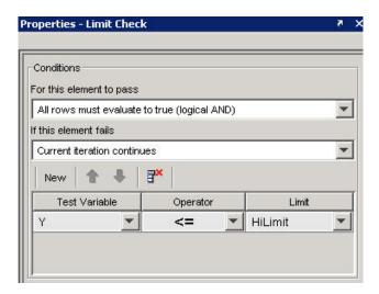
**6** To add another limit comparison operation, click the **New** button in the **Properties** pane. SystemTest adds a new row below the last limit you specified. In this new row, set **Test Variable** to Y, set **Operator** to >=, and set **Limit** to LowLimit.
