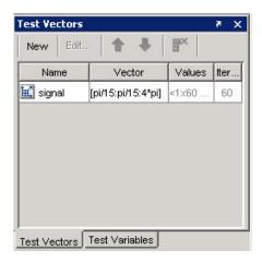
After you create the test vector, in the **Test Browser** pane, the **Iterations** section label updates to include the number of iterations defined by the test vector. It should say Iterations (60).
