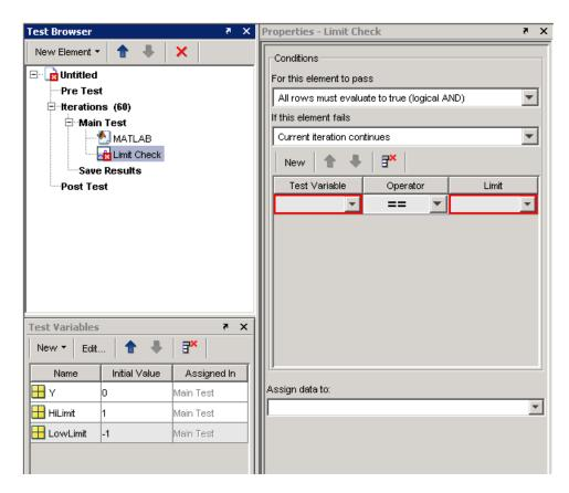
Notice that the Limit Check element icon in the **Test Browser** shows a red x, which indicates that information is missing. The corresponding red outlining in the **Properties** pane highlights any fields that require configuration.
