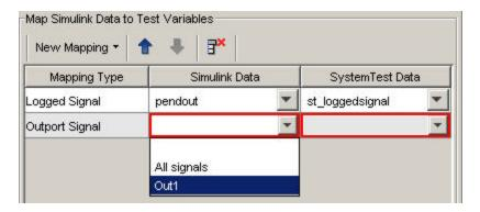
**3** Specify the SystemTest test variable to which you want to map the outport signals. Click the **SystemTest Data** field and select a test variable from the list. For this example, select **st\_outportsignal**.
