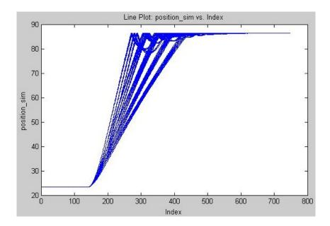
This output shows that the test results group in small clusters. You can use a constraint to see which of the test vectors cause this clustering.
