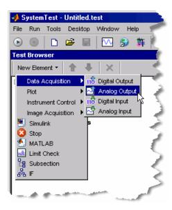
The new element appears in the browser tree, and its properties appear in the **Properties** pane. SystemTest scans your computer for installed data acquisition adaptors and devices. This can take several seconds.
