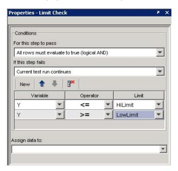
The following figure shows the configuration of this second limit:
