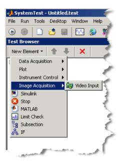
SystemTest adds the Video Input element to the Main Test section of the test and displays the **Properties** pane for the Video Input element. (You can also add elements to the Pre Test or Post Test sections of a test but this example does not require it.)
