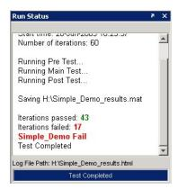
If your test includes a Plot element, SystemTest creates the plot and updates the plot during each iteration. Since Limit Check elements evaluate whether an iteration passed or failed, they directly affect the data that appears in the test execution log and the **Run Status** pane.
