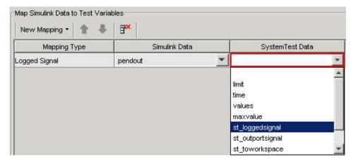
SystemTest creates the mapping to the test variable.
