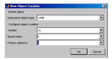
**10** Click **OK** to return to the Editing: Instrument1 dialog box, where the instrument object is now filled in and selected for this resource (GPIB0-5).
