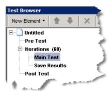
**2** Specify the element you want to add to the test section. For this example, click the **New Element** button and select **MATLAB**. SystemTest adds a MATLAB element to the Main Test section of your test and opens the MATLAB element property page in the **Properties** pane of the SystemTest desktop.
