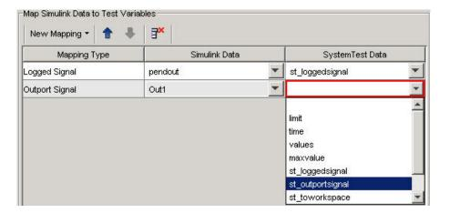
SystemTest creates the mapping to the test variable.
